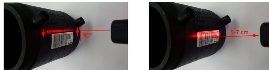
The red light band should be centered horizontally over the complete barcode. The barcode is not read in if the red light-band is in any other position. A successful reading of the barcode is signalled by sounding of a verification tone.
