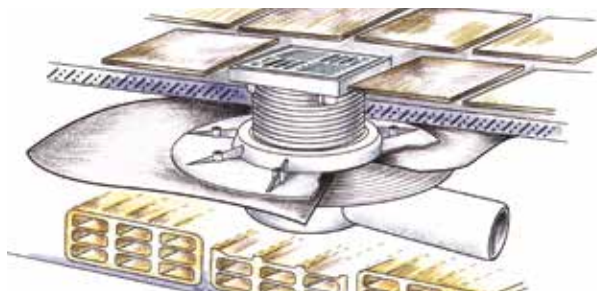
Example of installation with insulating membrane
