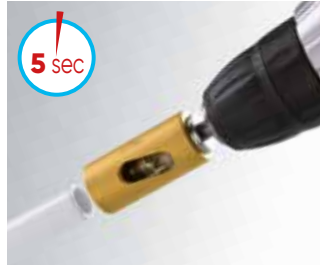
2- Chamfering the pipe
