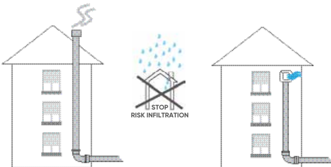
Example of a discharge ventilation system with ARIO next to a window.
