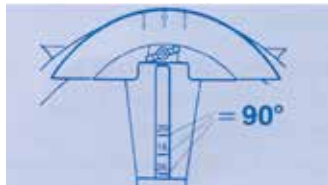
Phase 3 - Use the lever of the clamp until you reach the desired bending angle.
